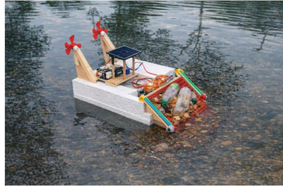
Figure 5. Experimental validation of the developed photovoltaic-powered water surface cleaning boat during field testing, showing active collection of floating debris under real lake environment.
