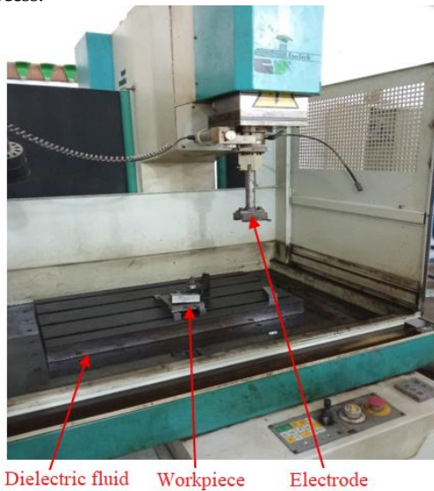
Figure 1. Experimental set up of EDM machine (EROTECH basic 450)
