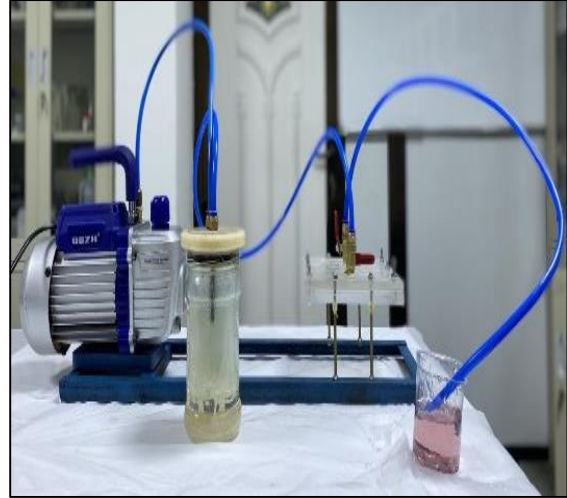
Figure 2. Vacuum casting mould of composite Samples
