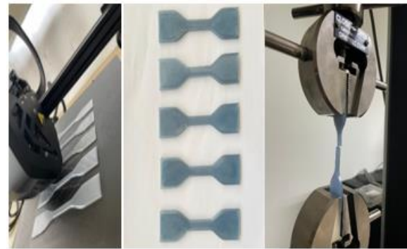
Figure 4. 3D prints tensile test specimen
