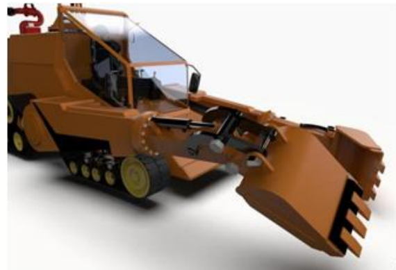
Figure 5. Rescue vehicle double digging grapple display
