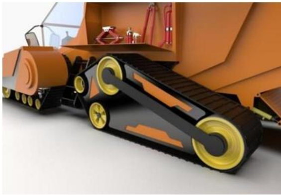
Figure 11. Rescue vehicle can lift wheelset details
