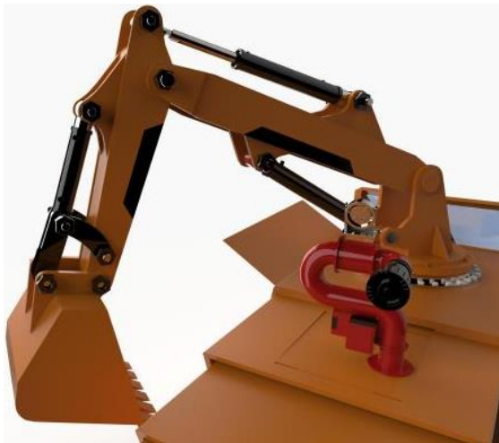
Figure 7. Rescue vehicle tail gouging arm display
