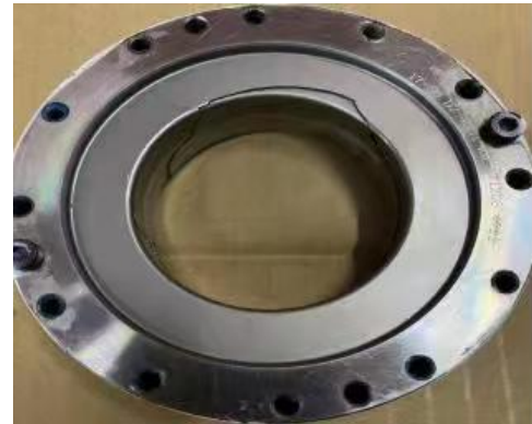
(a) Picture of tear at the bottom of flexible wheel cup
