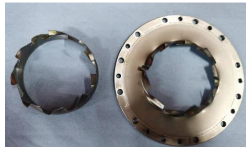
(b) Picture of tear at the root of flexible gear teeth
