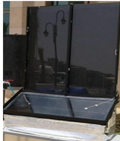
b. Stepped SS with vertical corrugated wick still
