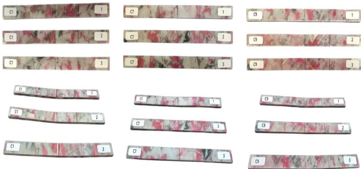
Figure 5. Before and after flexural testing
