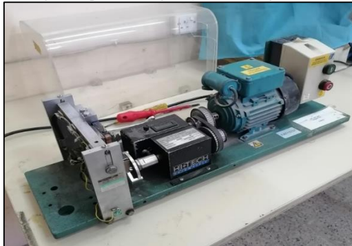
Figure 7. Bending-alternating fatigue device HSM20
