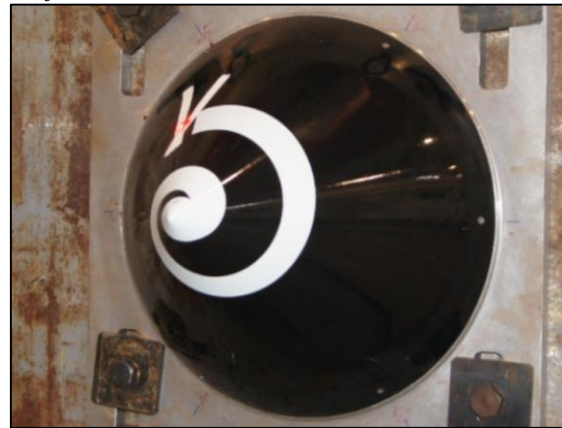
Figure 1. The cap cone of aircraft engine
