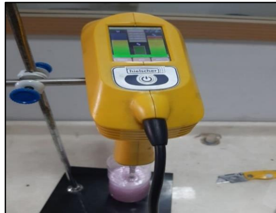
Figure 4. The device of the ultrasonic processor type UP200Ht
