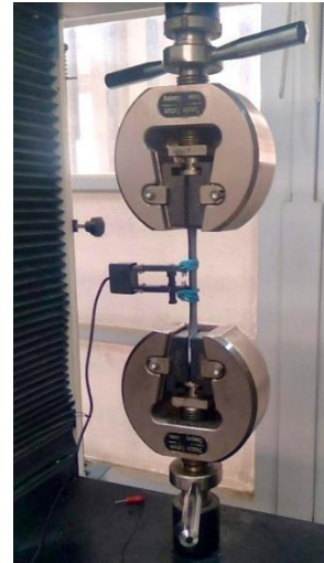
Figure 2. Experimental set-up of tensile test
