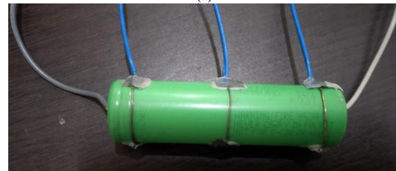
Figure 2. Thermocouple arrangement over cell surface (a) schematic layout, (b) pictorial view
