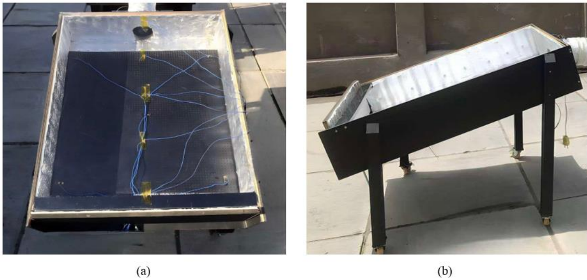
Figure 3. Photographs of the solar air collector: (a) Top view, (b) Side view.
