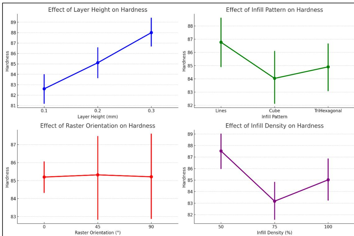
Figure 4. Main effect plots for hardness
