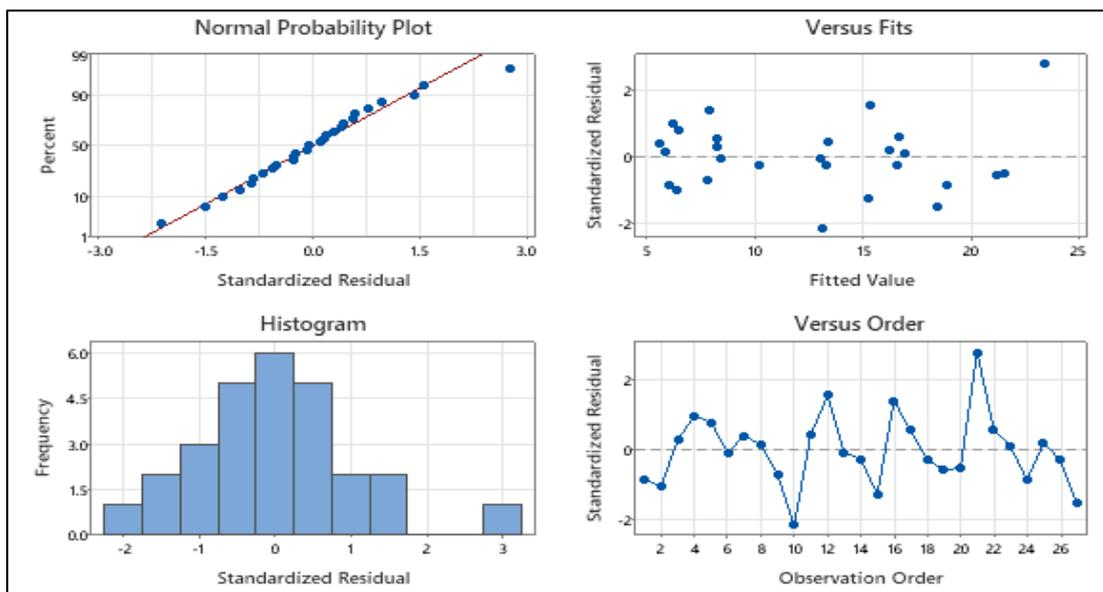
Figure 7. Residual Plots for Compressive Strength
