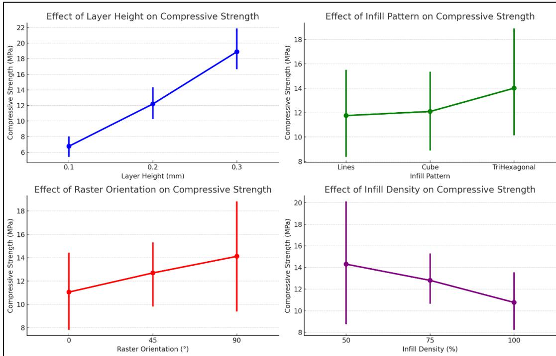
Figure 5. Main effect plots for compressive strength
