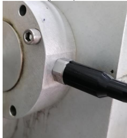
Figure 4. An accelerometer mounted on SQ WTS
