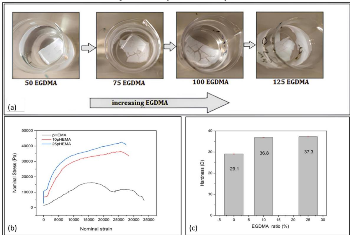
**Figure 3.** (a) Digital images of pHEMA: The effect of EGDMA concentration on AM (b) Stress - strain curves (c) Surface hardness
