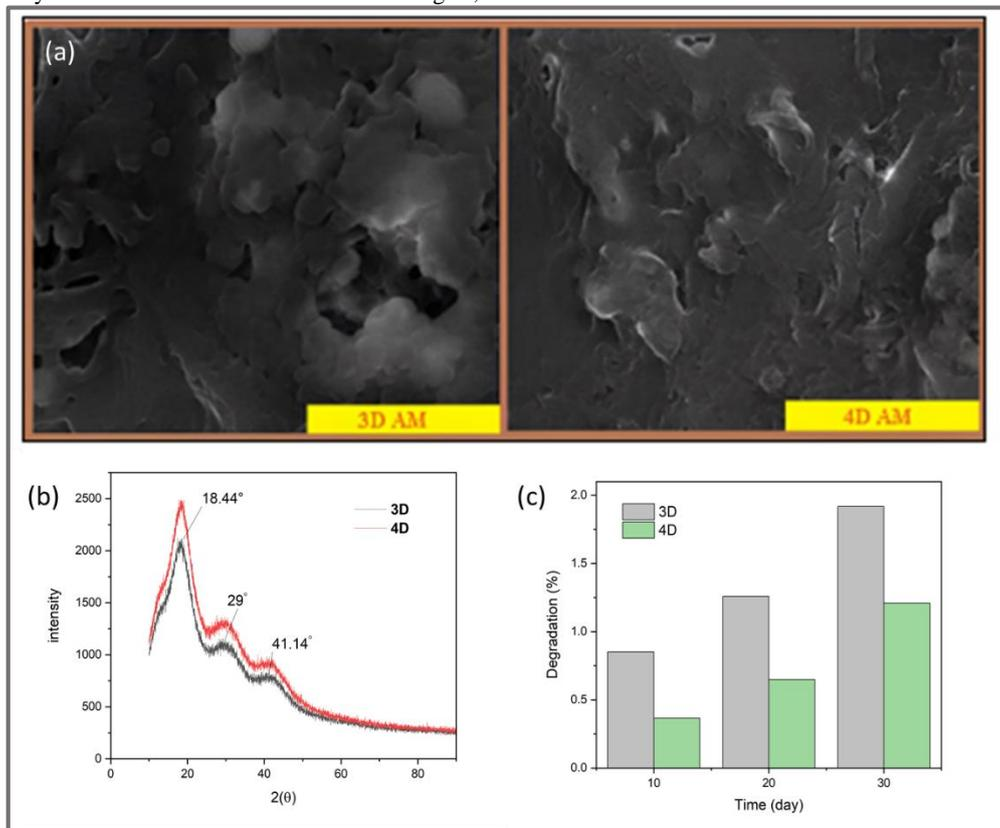
**Figure 4.** Comparison of physicochemical characterization of pHEMA produced by both 3D and 4D: (a) SEM micrographs (x35magnification), (b) XRD pattern and (c) Hydrolytic degradation
