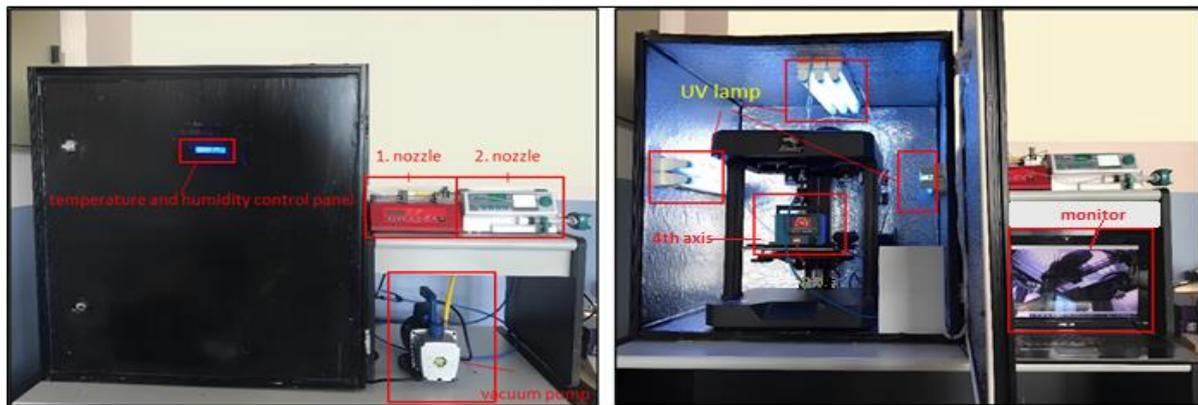
**Figure 1.** Integrated 4D additive manufacturing system with UV-photopolymerization
