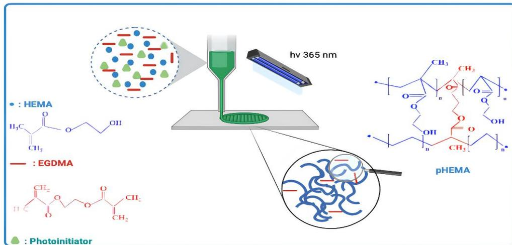
**Figure 2.** Schematic presentation of AM of pHEMA
