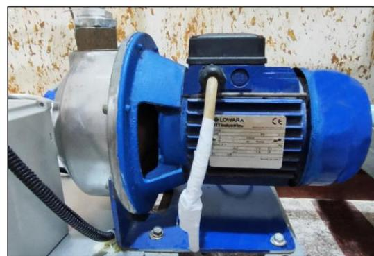
Figure 1. Centrifugal pump type CEA 210/2.
