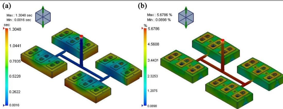
**Figure 3.** Filling time (a) and volumetric shrinkage rate (b) of model 01
