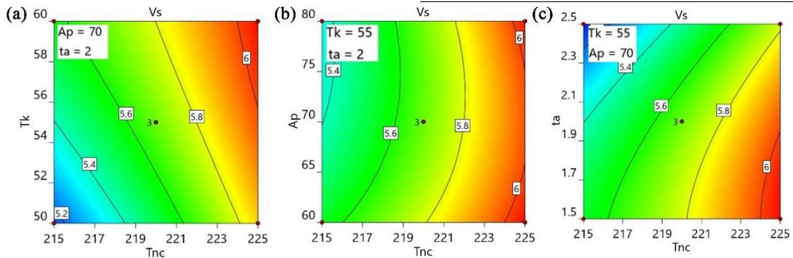
Figure 7. Contour plot for the influence of process parameters on  $V_s$
