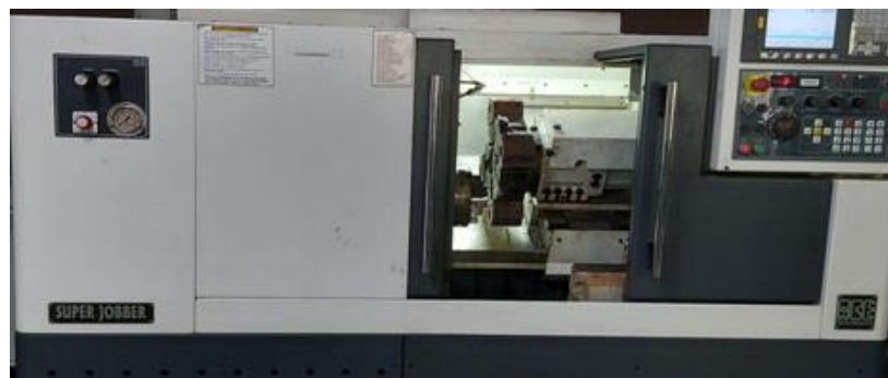
Figure 1. CNC Fanuc configured Super Jobber makes computer numerical controller turner machine.
