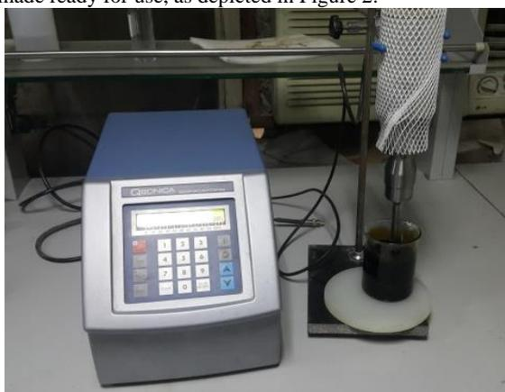
Figure 1. Nano Mixture Stirrer (SonicatorsQsonica. LLC) device
