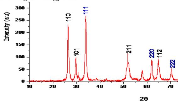
Figure 3. XRD pattern of Nanocomposite ( PVP: CNTs ) mixture
