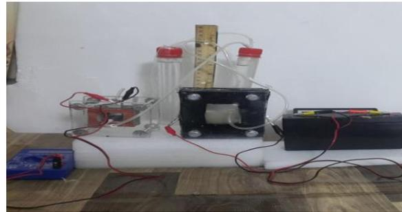
**Figure 5.** Show electrolyser cell and fuel cell system
