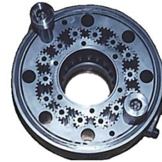
Figure 1. The physical picture of 6-8 type non-circular gear hydraulic motor[17]
