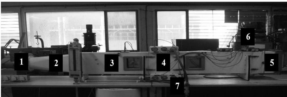
1.Centrifugal fan 2.Conical section 3. Calming section 4.Test section 5. Honey combs 6.Measurements (Thermocouples , Watt meter) 7. Pressure gauge
