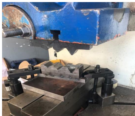
Figure 4. a. Connecting the die to the press with an adapter piece b. Measurement of springback in a laser optical projector.
