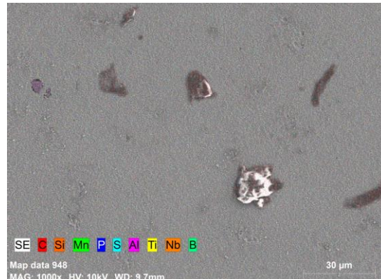
Figure 3. a. Microstructure of material SCGADUB1180 b. Elemental distribution of material SCGADUB1180
