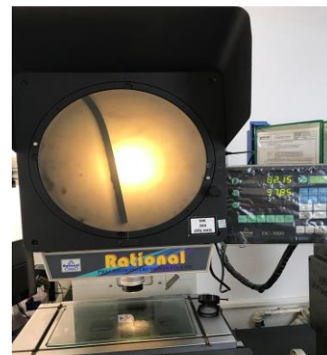
Figure 4. a. Connecting the die to the press with an adapter piece b. Measurement of springback in a laser optical projector.
