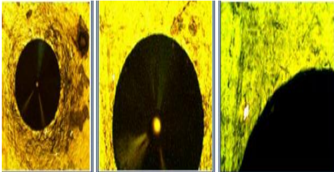
Figure 15. Rockwell type - C test for sputtered samples with Ag at 2 hrs.
