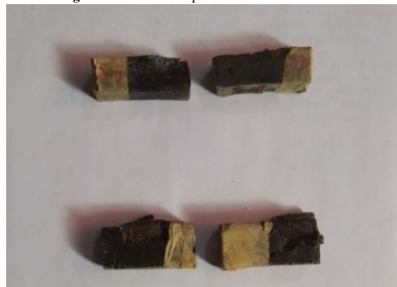
Figure 20. Fractured specimen from impact test
