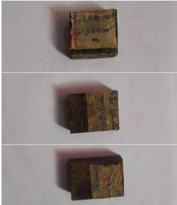
Figure 21. Fractured Specimen from hardness test evaluation
