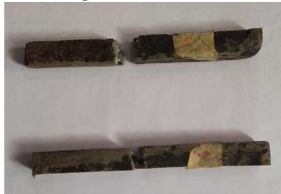
Figure 19. Fractured specimen from tensile tests
