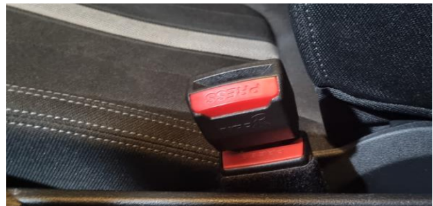
Figure 6. Implementation of a product for canceling seat belt alarms and the possibility of plugging it.
