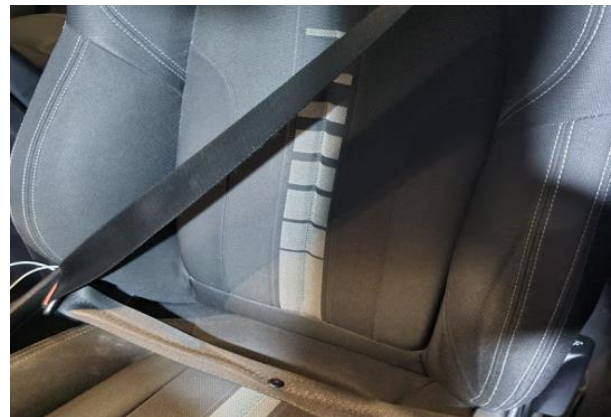
Figure 5. Method to cancel alarm of seat belt by placing behind back
