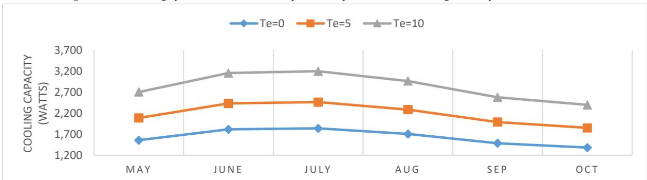
Figure 8. ECR cycle cooling capacity for different evaporator temperatures and the average monthly solar radiation.
