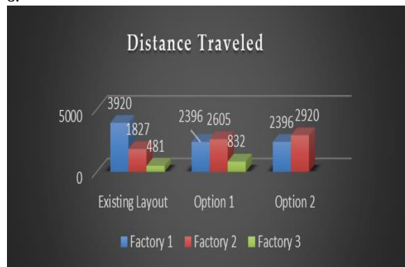
Figure 8. The distance travelled by the forklifts in the three layouts
