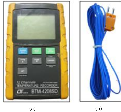
Figure 4. Measuring instruments: (a) data logger, (b) type-K thermocouple.
