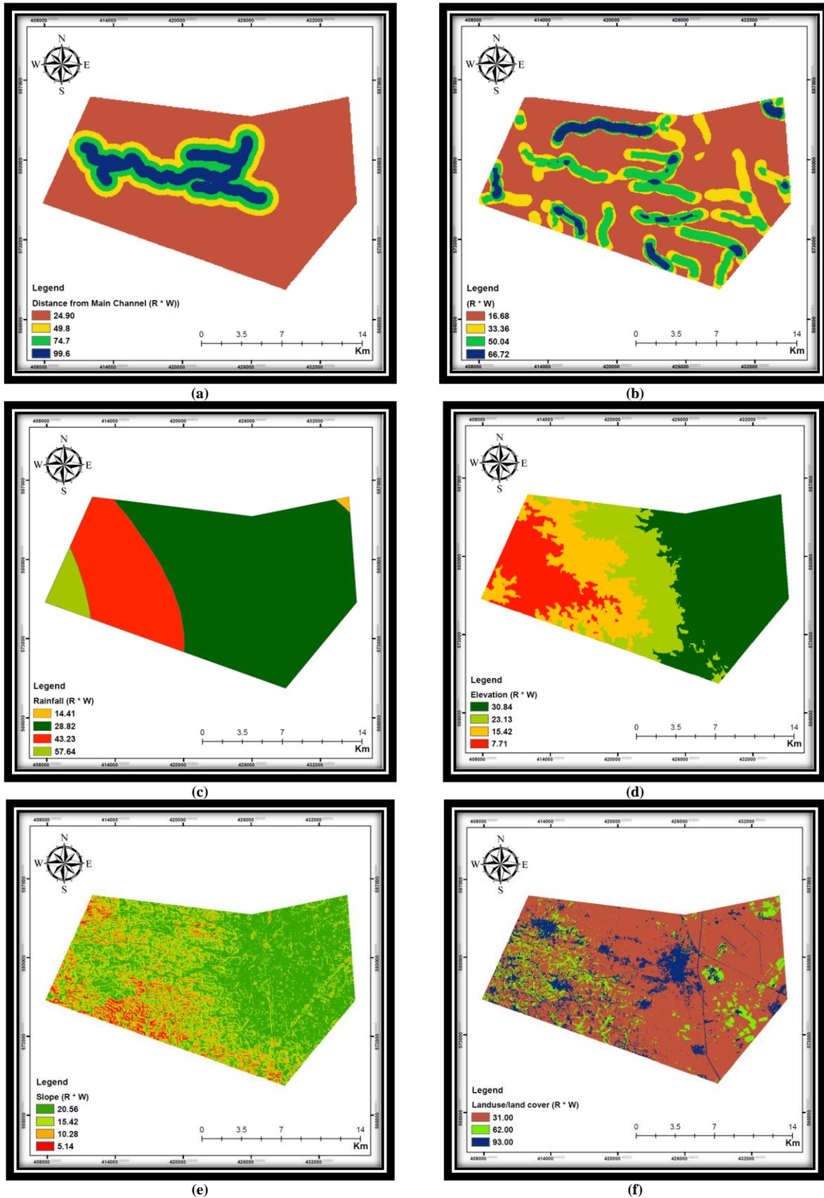
**Figure 3.** (a) Distance from Main Channels; (b) Drainage Density; (c) Rainfall; (d) Elevations; (e) Slope; (f) Land cover/land use maps.
