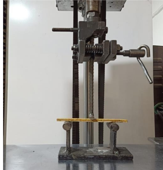
Figure 5. Flexural test setup
