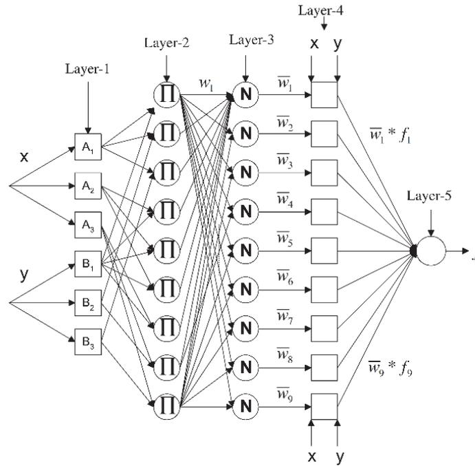
Figure 3. ANFIS two-input one output structure
