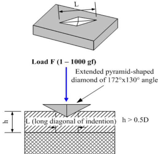
Figure 4. Knoop Hardness Test
