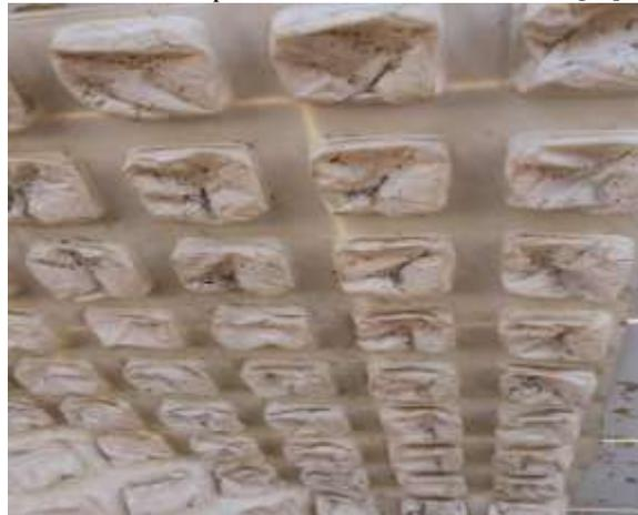
**Figure 3.** Pasting PCM on the PV panels backside.
