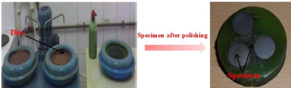
Figure 5. Test specimen polishing on disc abrasive
