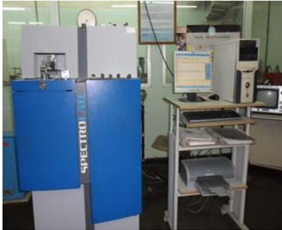
Figure 1. Emission spectrometry
