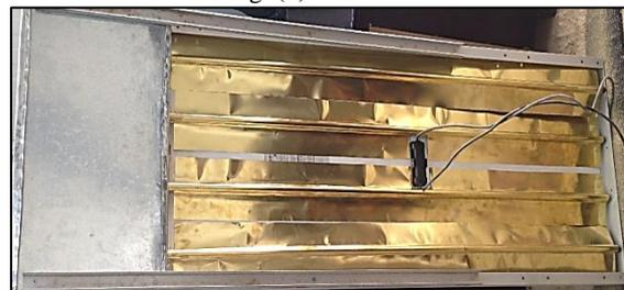
Figure 2. copper plate with heat pipe in the back of panel.
