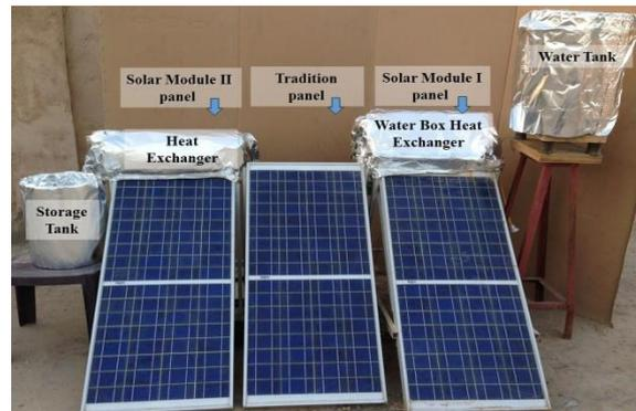
Figure 1. Experimental setup system.
