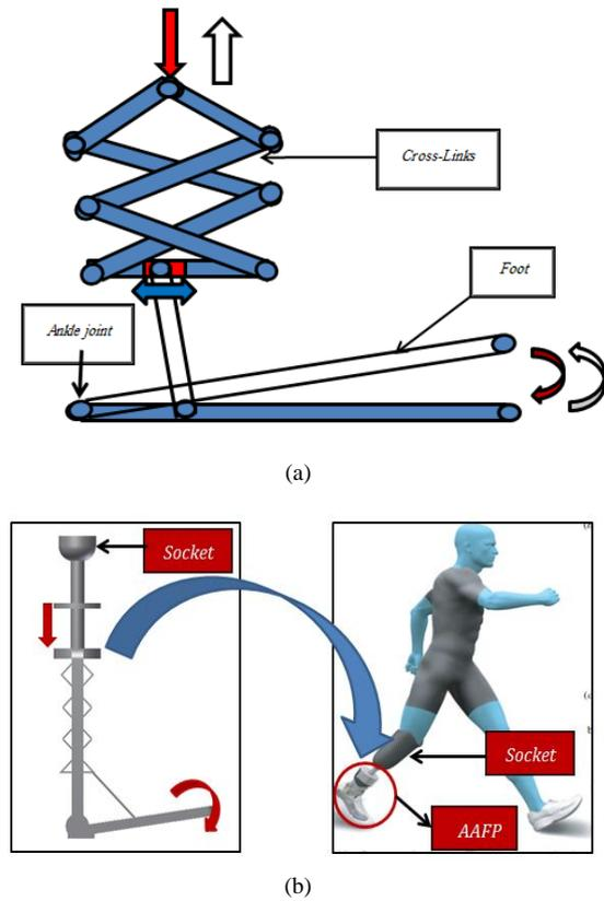
**Figure 4.** Ankle-Foot Prosthetic. (a) Mechanism of Prosthetic animation (b) Connection AAPF to socket.
