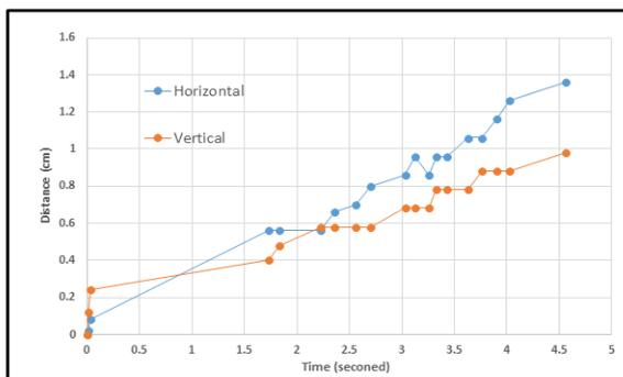
Figure 11. Movement of pin A in cartesian coordinate.
