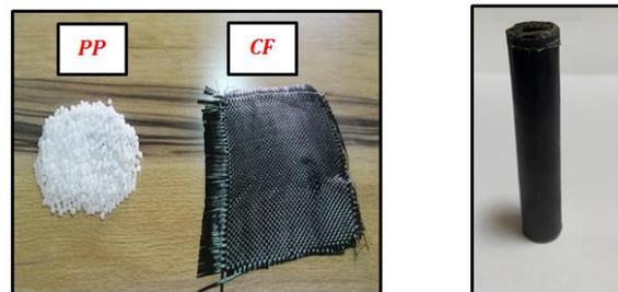
**Figure 7.** CFRP Specimen.
