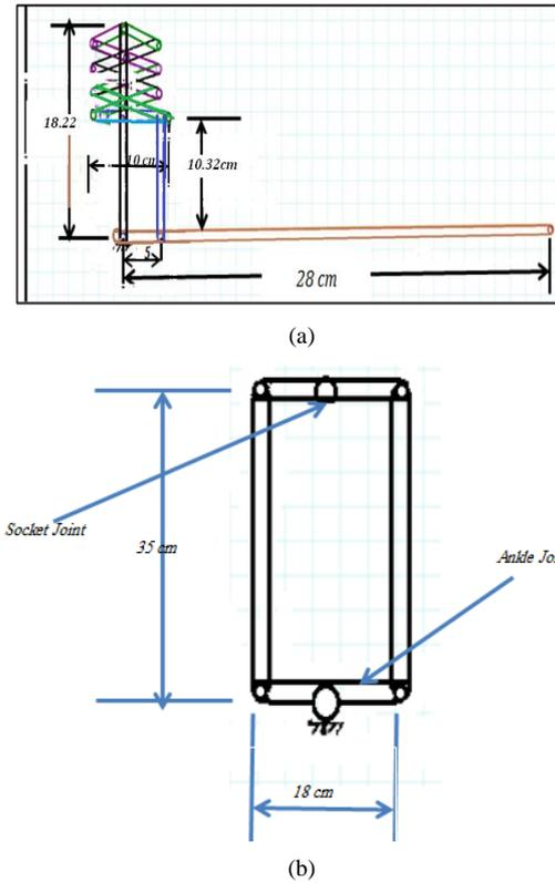
**Figure 3.** Dimensions of articulated prosthetic lower limb. (a) Front view, (b) Side view
