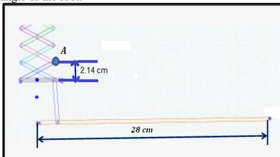
Figure 10. Null position of a prosthetic foot.
