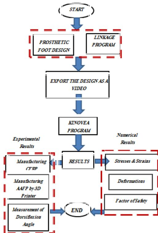
Figure 2. Flow chart of the current work.
