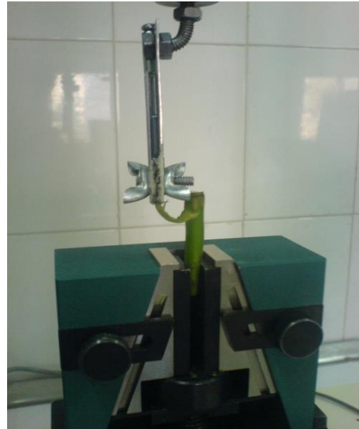
Figure 2b. Device to hold and connect the leaf to UTM for picking force measuring
