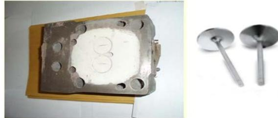
Figure 2. PSZ coated cylinder head and valves
