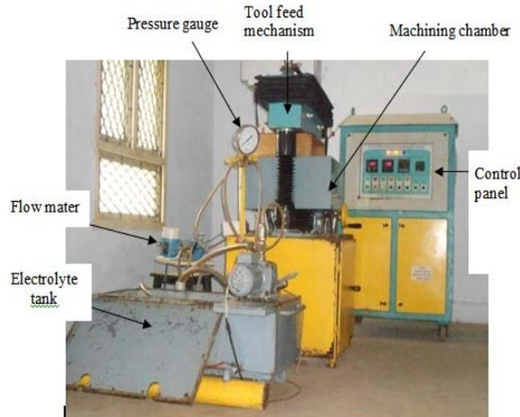
**Figure 2.** Electrochemical machining set-up
