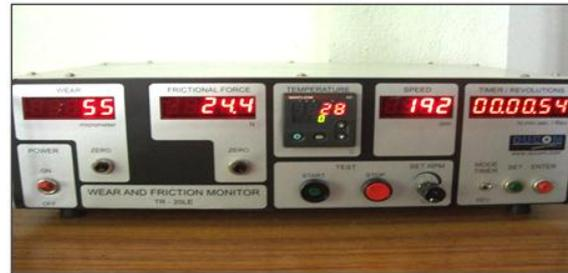
Figure 2: Controller of the wear and friction-testing machine.
