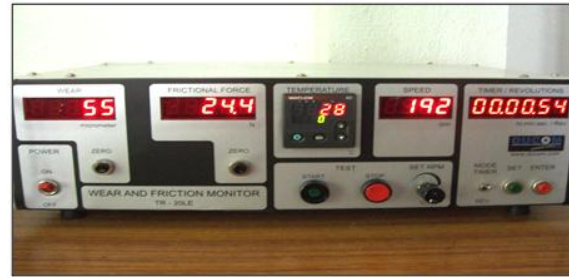
Figure 2: Controller of the wear and friction-testing machine.
