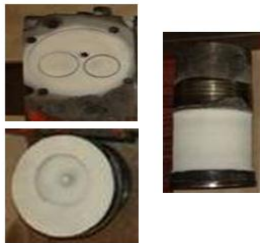
Figure 1: Photographic view of 60EPCY 20PI coated piston, cylinder head with valves and liner.
