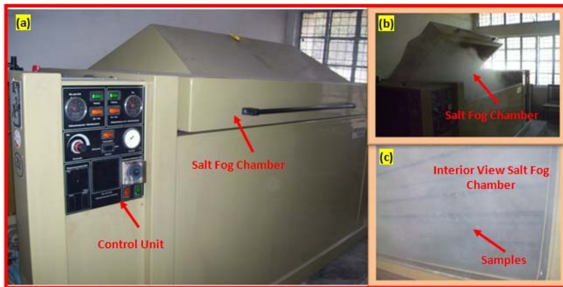
Figure 1: Experimental set-up for Salt spray (Fog) testing (a) Salt fog testing set up, (b) Salt fog chamber, (c) Interior view of chamber.
