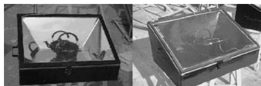
Figure 1 Tested solar cookers: a) Black painted box type cooker, and b) Mirrors box type cooker
