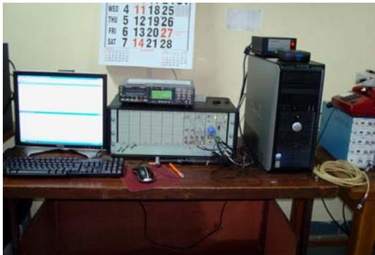
Figure 5 Four channel data-acquisition system
