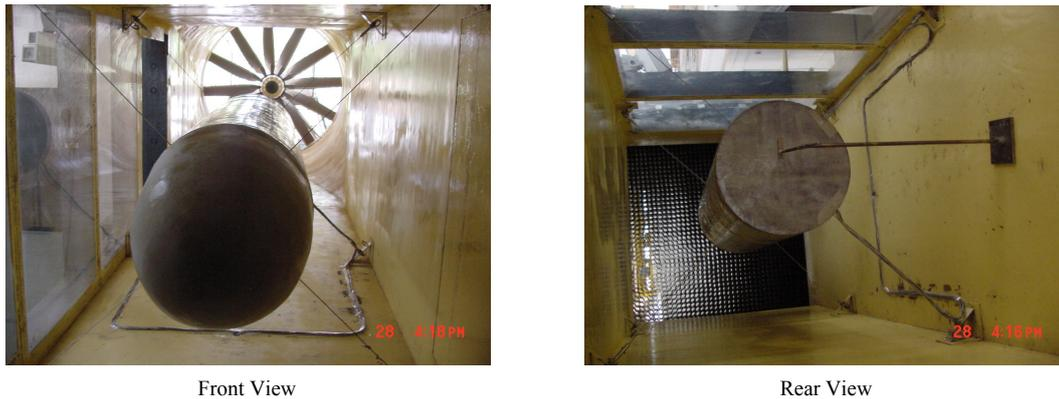
Figure 9: Ellipsoidal Model of 2.3:1 major to minor axes ratio mounted in the test section
