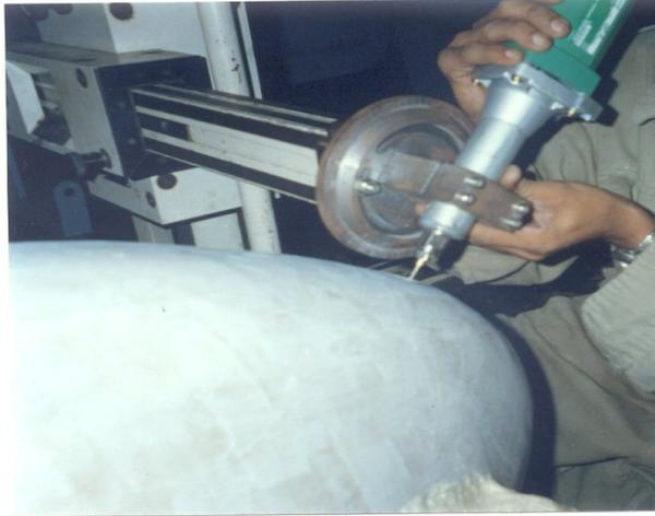
Figure 6: Drilling of pressure holes on the model
