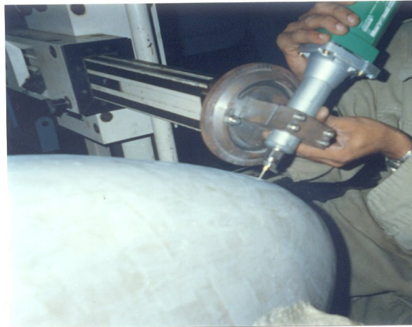
Figure 6: Drilling of pressure holes on the model
