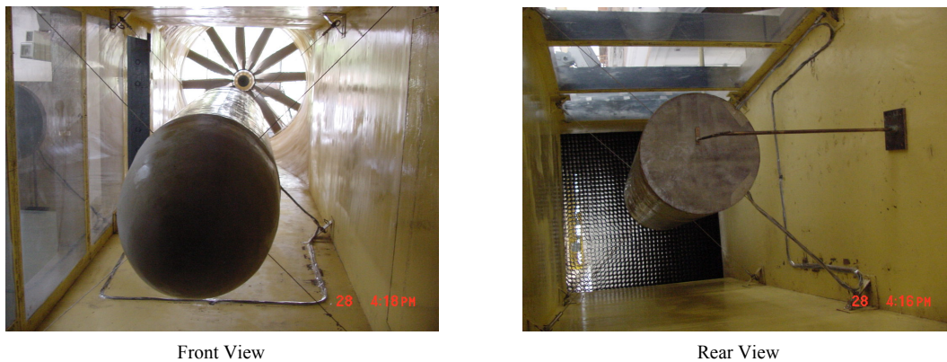
Figure 9: Ellipsoidal Model of 2.3:1 major to minor axes ratio mounted in the test section
