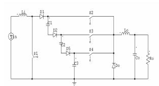
Fig 4. The 3-Stage non-inverting Cuk converter
