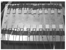
Plate 2: TEC modules attached to heat sink
