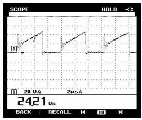
Figure 6 Measured voltage across MOSFET S1
