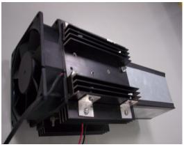
Plate 1: A pre-developed TEC cooling prototypes.
