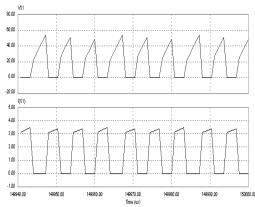
Figure 7 Simulation waveforms of MOSFET switch S1
