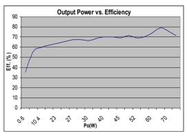
Figure 10 Output power versus efficiency
