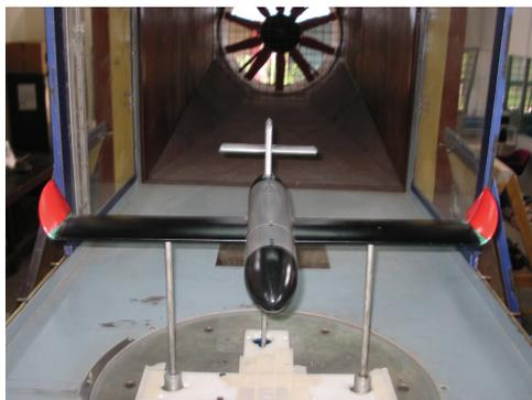
Figure 5: Aircraft model check for 0° angle of attack.
