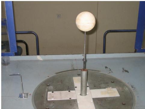
Figure 7: Sphere model mounted in wind tunnel test section
