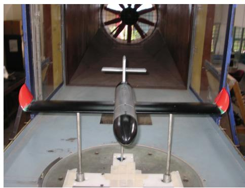
Figure 5: Aircraft model check for 0° angle of attack.
