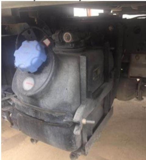
Figure 13. optimization scheme of urea box bracket
