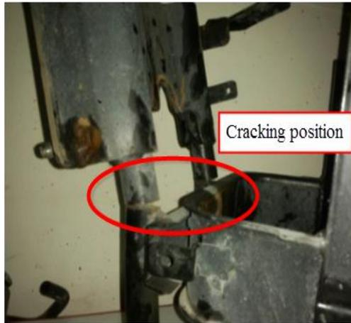
Figure 1. Cracking of urea box bracket
