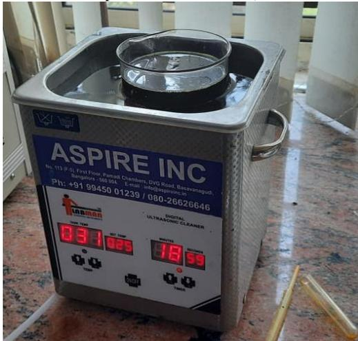
Figure 2. Biodiesel subjected to ultrasonication
